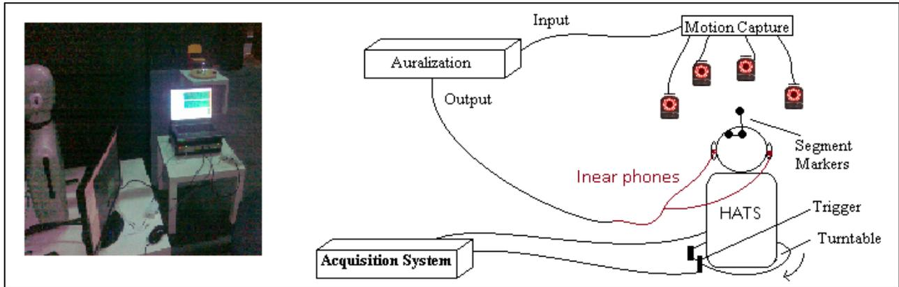
Figure 2 - Test-bed for measuring end-to-end delay
