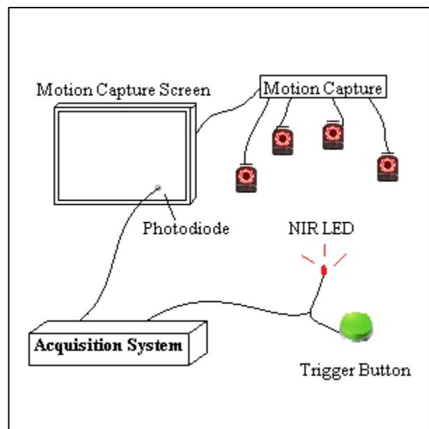
Figure 1 - Test-bed for tracking internal latencies
