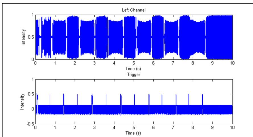
Figure 4 - Result example from end-to-end delay measurement
