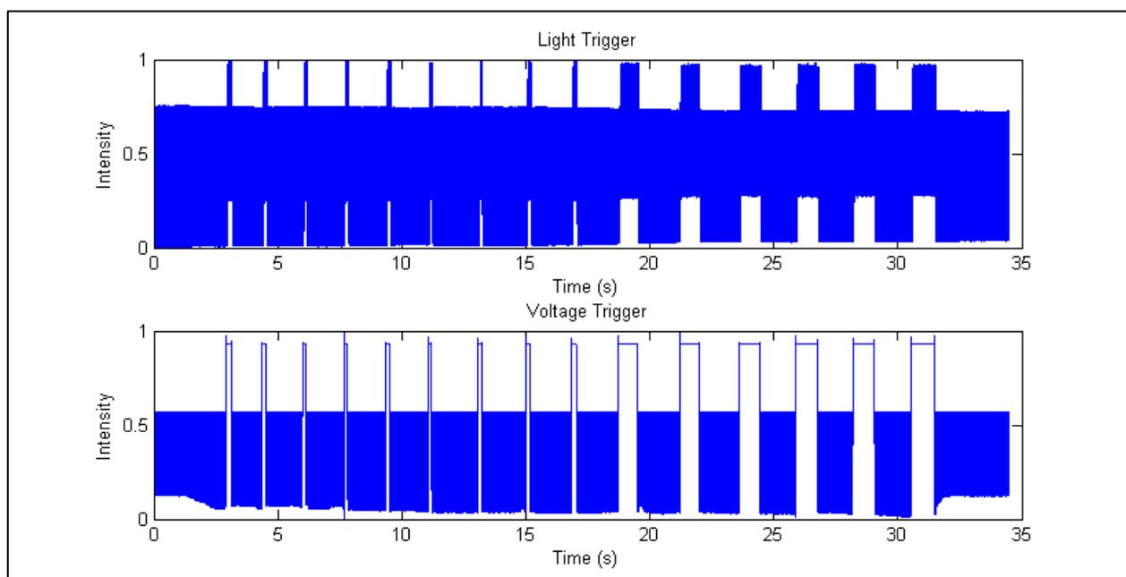
Figure 3 – Acquisition result from test-bed for tracking internal latencies
